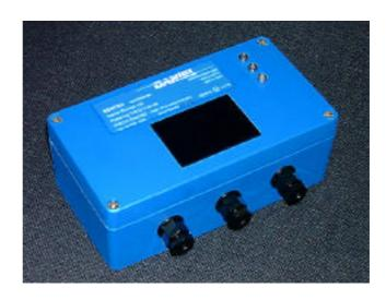
the RS-485 serial data point whereby up to 64 Sentry barriers can be chained together and connected to a single control port on the host. The Sentry can also communicate via a Mercury terminal.
